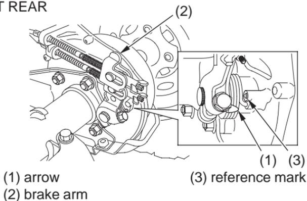
1. Apply the brake control and check the movement of the arrow (1) on the brake arm (2).
