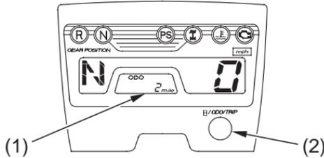
(1) odometer (2) hourmeter/odometer/tripmeter select button
