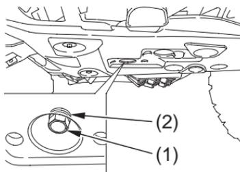
(1) engine oil drain plug      (2) sealing washer
