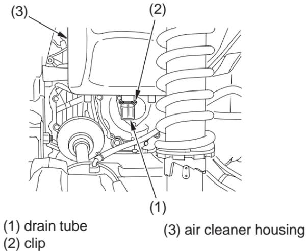
1. Remove the drain tube (1) by removing the clip (2) under the air cleaner housing (3).
