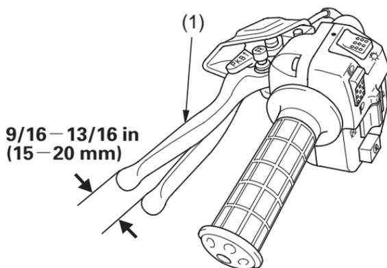
(1) rear brake lever/parking brake lever
