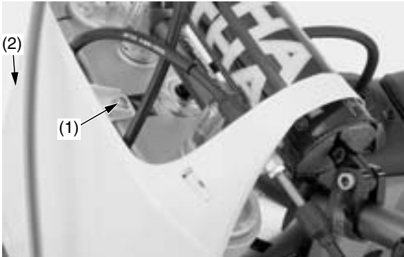
(1) number plate bolt (2) number plate
